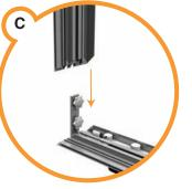
Connect the corners using the pre-installed CSS connectors and thumb screws provided.
