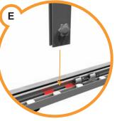
Locate the 'insert vertical here' sticker and secure the central column to the frame using the CBX connectors.
