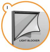
Lightblocker fabric is applied to the rear of the unit using velcro.
