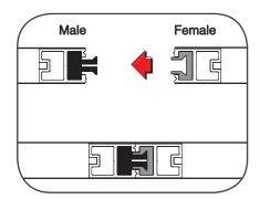
All panels have male and female connectors. The male connector should connectors down over the male always be on your right when facing the connectors. front of the display.
