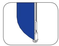
The base level has adjustable feet that allow you to level the display on an uneven floor. You should assemble the entire base level before adjusting
